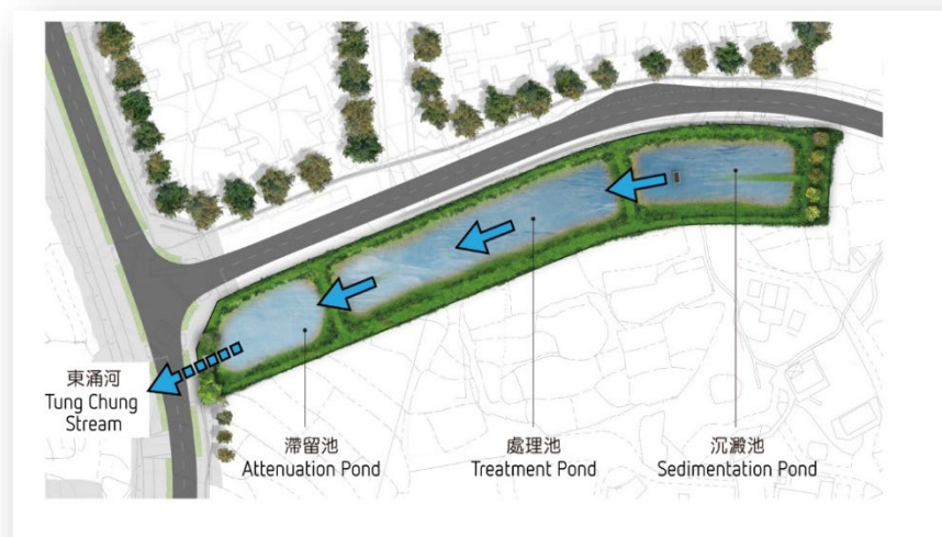
可持續城市排水系統構想圖 Sustainable urban drainage system conceptual design
